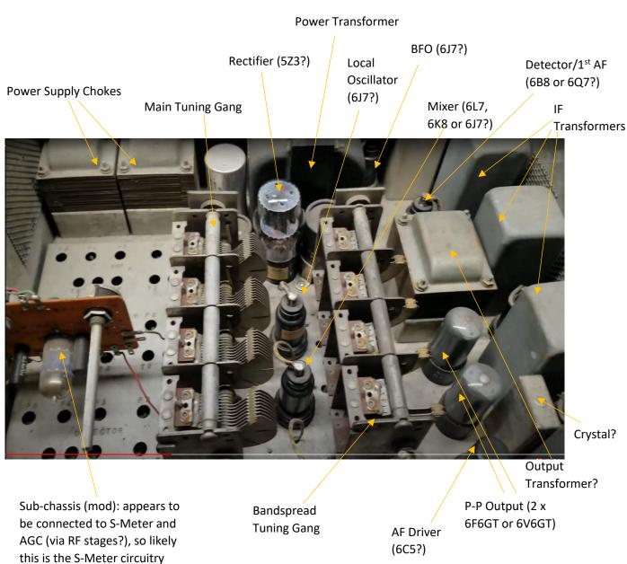
Implied tube line-up: 2 x RF amplifier stages (6SK7s?), mixer (6L7 or 6J7?), local oscillator (6J7?), 3 x IF amplifier stages (3 x 6K7?), 1st AF/detector (6B8 or 6Q7?), BFO (6J7?), AF Driver (6C5?), push-pull output (2 x 6F6 or 6V6?) and rectifier (5Z3?). It may have had an eye tube in place of the S-Meter originally also. If this is the line-up, it is quite a bit more sophisticated than the CSR-5 and the SMR-3 circuits.
